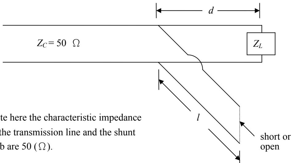
4. Find the expression of the input impedance,  $Z_{in}$ , for a cascaded transmission line shown in figure. If  $R_L$  is a pure real value and the  $\lambda$  is the guided wavelength of the wave propagated in all the
